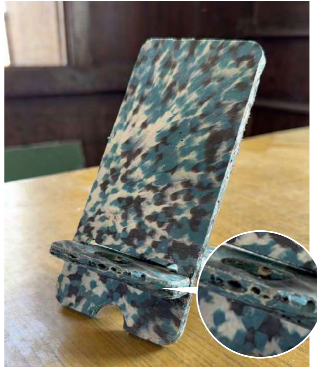
Figure 106 Paramendo phone stand prototype and a close-up image of the bubble inside
