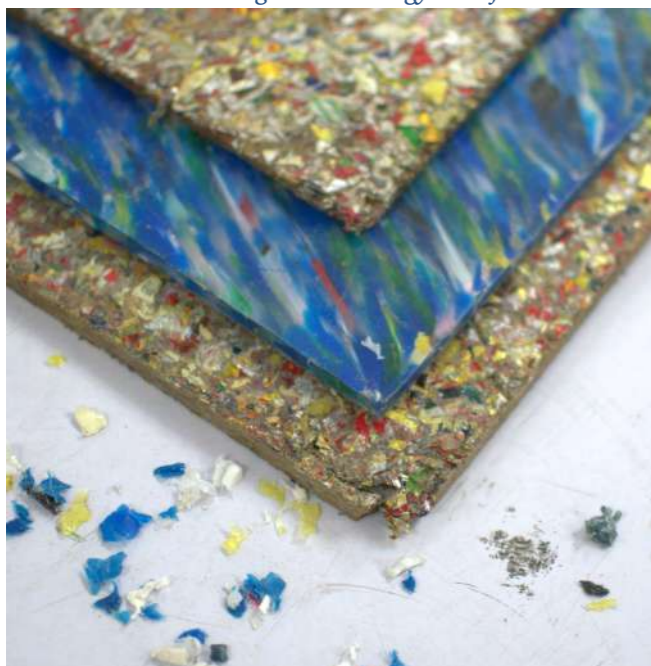
Figure 82 MLP & HDPE boards produced at Ree hub
