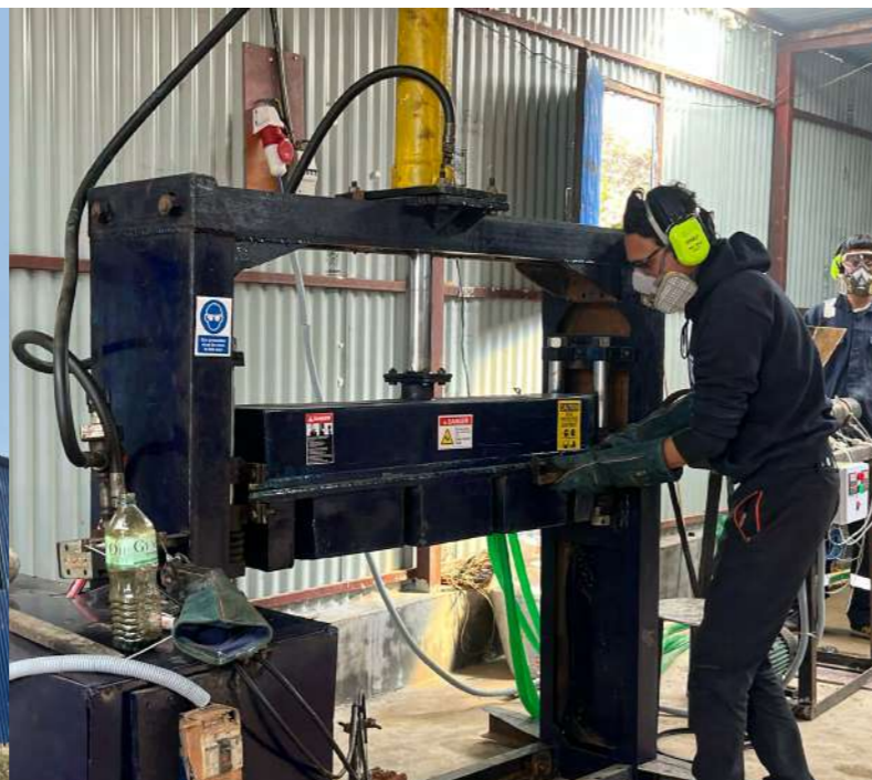
Figure 97 Decking machine in operation at Nagarjun Hub
